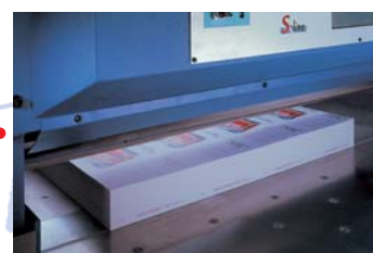
Before the cut: The material is placed in position. The front table is still closed.
