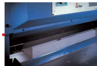
The waste removal process is activated. The front table is opened and the plexiglass plate is lowered.
