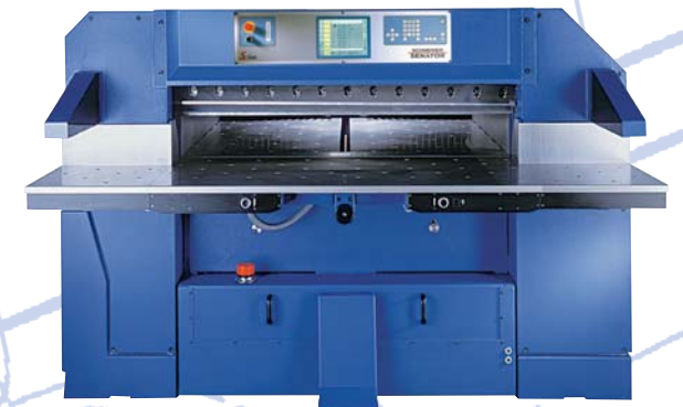
Ideally suited for the optional TrimmMaster System: the fully hydraulic Senator 137 H.
