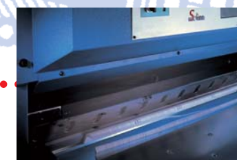
Cut – the waste paper falls into the gap.
