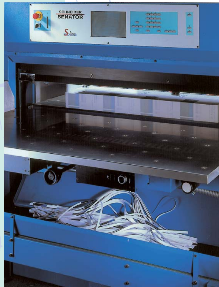
Senator TrimmMaster: Fast waste removal thanks to the front table opening.
