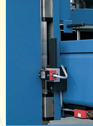
Virtually wear-free precision guide-rails
